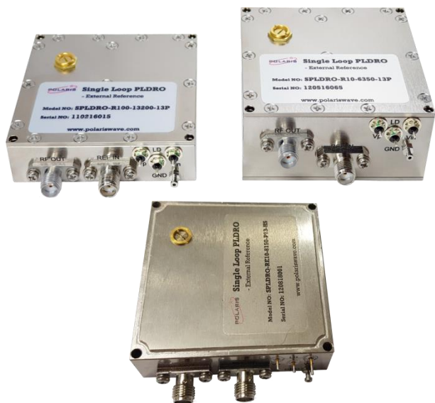
Single Loop PLDRO without Frequency Multiplier
