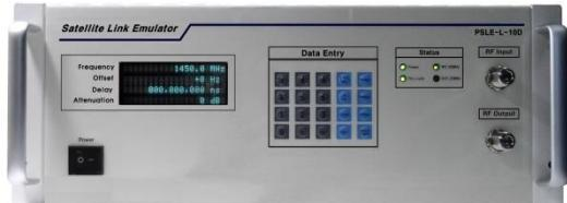
The PSLE-L-10D provides accurate simulation of propagation delay, path loss, and Doppler frequency shift for closed-loop testing of geostationary satellites and earth station terminals. The PSLE-L-10D operates from 950MHz to 1,450MHz and provides up to 10MHz bandwidth.
