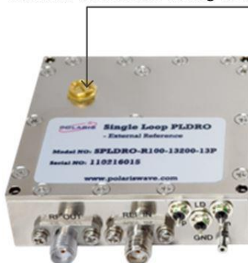
[Figure 2] Screw location of microwave tuning element screw
