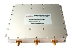
The Polaris DDS-2CH-OCXO is a dual channel direct digital synthsizer that provides ultra-precise frequency resolution, low spurious, and low phase noise performance. The DDS-2CH-OCXO has an internal 100MHz OCXO for excellent temperature stability of the system clock.
