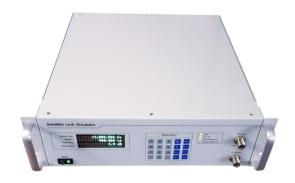
The ASLE-140-36D provides accurate reproductions of propagation time delay, path loss, and doppler frequency shift for closed-loop testing of geostationary satellites and earth station terminals. The ASLE-140-36D operates at 140 MHz and provides operating bandwidth of 36 MHz.
