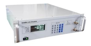
The ASLE-L-200D provides accurate reproductions for propagation time delay, path loss, and doppler frequency shift for closed-loop testing of geostationary satellites and earth station terminals. The ASLE-L-200D operates from 950 MHz to 1450 MHz and provides operating bandwidth of 200 MHz.
