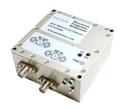
The PMFS-P synthesizers are a high power fixed frequency synthesizers that output RF power up to 20 dBm.
