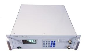
The ASLE-140-36D provides accurate simulation of propagation delay, path loss, and Doppler frequency shift for closed-loop testing of geostationary satellites and earth station terminals. The ASLE-140-36D operates at 140MHz and provides up to 36MHz bandwidth.
