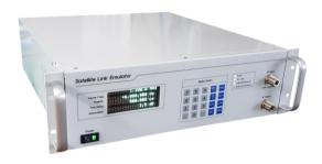
The ASLE-L-200D provides accurate simulation for propagation delay, path loss, and Doppler frequency shift for closed-loop testing of geostationary satellites and earth station terminals. The ASLE-L-200D operates from 950MHz to 1,450MHz and provides up to 200 MHz bandwidth.
